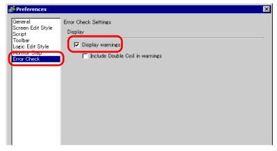
2 To start the error check, from the [Project (F)] menu, point to [Utility (T)] and select [Error Check (E)].
