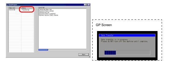
7 When the transfer finishes, the status changes from [Transferring] to [Complete Transfer]. Click [Close].
