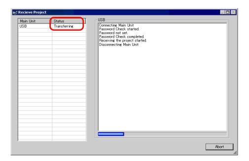
5 When the transfer finishes, the status changes from [Transferring] to [Complete Transfer]. Click [Close].
