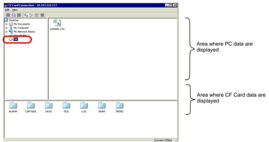
4 Select the Recipe data (ZR00000.csv) from the data displayed on the right-hand side, then drag it to the lower CF Card area.
