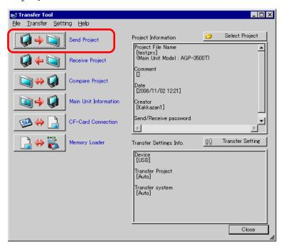
The following dialog box appears during transfer to check the communication status. During the transfer, the GP changes to Transferring mode and communication with the device/PLC is suspended.
