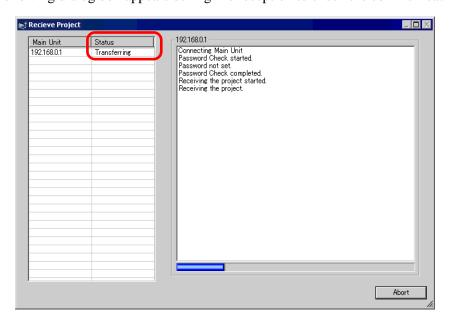
5 When the transfer finishes, the status changes from [Transferring] to [Complete Transfer]. Click [Close].
