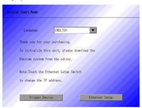
This screen will appear when you first connect the GP's power cord. After transferring a project once, this screen will not appear.
