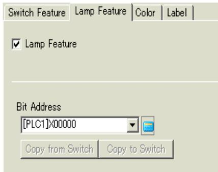
When using multiple bit addresses or Word addresses, click [Details]. Specify the operation condition and bit addresses for the lamp.
