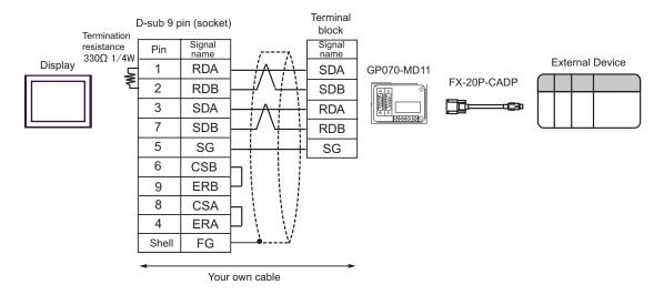
C) When using the online adapter (CA4-ADPONL-01) by Pro-face, the 2-port adapter cable for AGP (CA3-MDCB11) by Pro-face, the 2-port adapter II (GP070-MD11) by Pro-face, and the connector conversion cable (FX-20P-CADP) by Mitsubishi Electric Corp.
