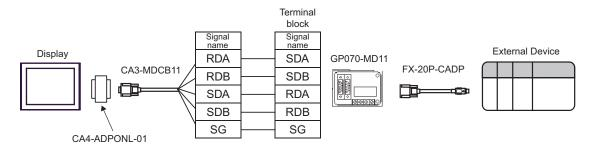
D) When using the online adapter (CA4-ADPONL-01) by Pro-face, your own cable, the 2-port adapter II (GP070-MD11) by Pro-face, and the connector conversion cable (FX-20P-CADP) by Mitsubishi Electric Corp.
