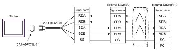
Do not connect the FG terminal of CA3-CBL422-01 to the External Device.
