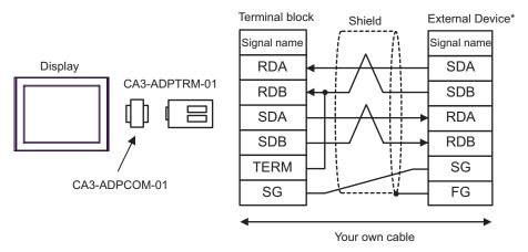
\* Turn On the termination resistance switch of the External Device, and set the operation mode to 3.
