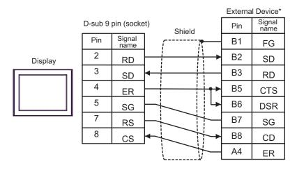
\* Set the operation mode on the External Device interface to 1.
