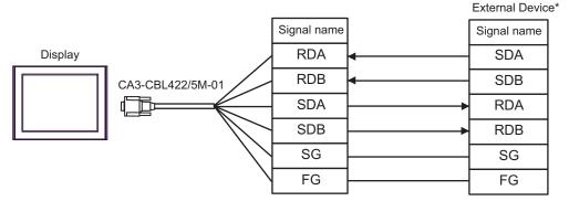
\*Turn On the termination resistance switch of the External Device, and set the operation mode to 3.
