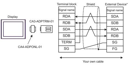
\* Turn On the termination resistance switch of the External Device, and set the operation mode to 3.
