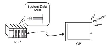
You can sound the GP internal buzzer from a device/PLC. You need to set the GP's system data area to the PLC to sound the buzzer.
