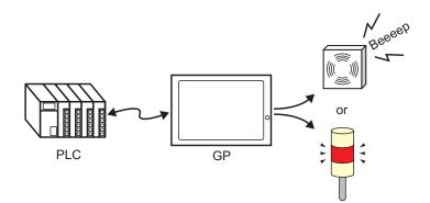
The output to sound an external buzzer is provided with the GP's AUX terminal.
