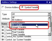
**3** Only addresses that match the [Bit Variable] type are displayed in the list. Drag the address "Start" to the terminal being mapped.
