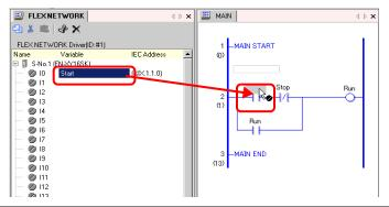
2 The address will be mapped and the I/O address (IEC address) will be displayed.
