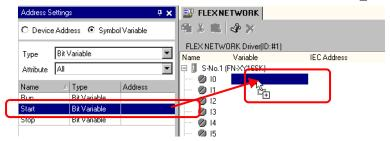
4 The address will be mapped and the I/O address (IEC address) will be displayed.
