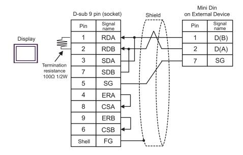
C) When using the online adapter (CA4-ADPONL-01), the connector terminal block conversion adapter (CA3-ADPTRM-01) by Pro-face and your own cable
