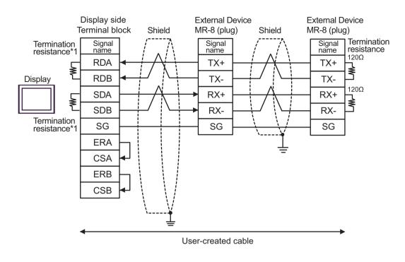
• When the External device has the SG terminal, connect it to the SG terminal of the Display.
