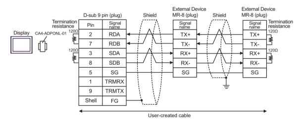
**NOTE** • The cable length must be 300m or less.
