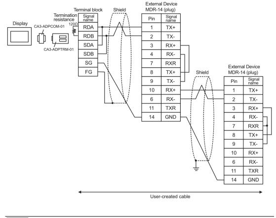
**NOTE** • The cable length must be 300m or less.
