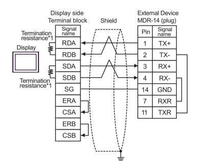
\*1 The resistance in the Display is used as the termination resistance. Set the value of the DIP Switch on the rear of the Display as shown in the table below.
