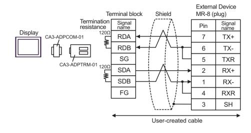
**NOTE** • The cable length must be 300m or less.
