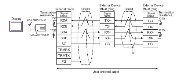
• When the External device has the SG terminal, connect it to the SG terminal of the Display.
