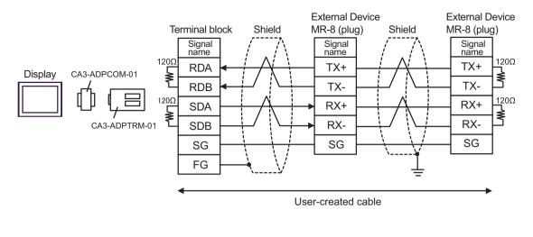
• When the External Device has the SG terminal, connect it to the SG terminal of the Display.• The cable length must be 300m or less.
