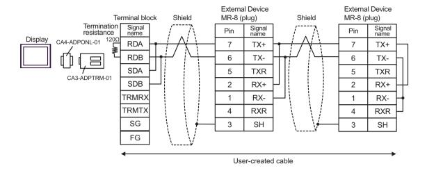
**NOTE** • The cable length must be 300m or less.
