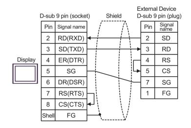
• The cable length must be 15m or less.
