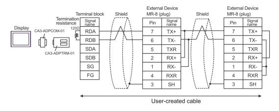
**NOTE** • The cable length must be 300m or less.
