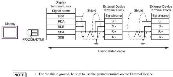
Turn on the termination resistor switch on the External Device.
