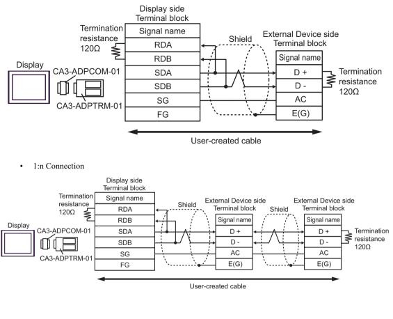
• On the final External Device, turn on DIP Switch S2 to apply termination resistance of 120  $\Omega$ 1/2 W.
