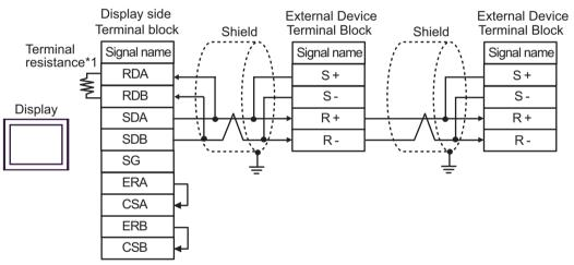
• For the shield ground, be sure to use the ground terminal on the External Device.
