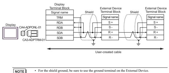
• Turn on the termination resistor switch on the External Device located at the end.
