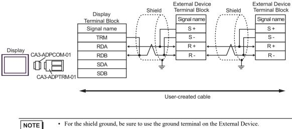
• Turn on the termination resistor switch on the External Device located at the end.
