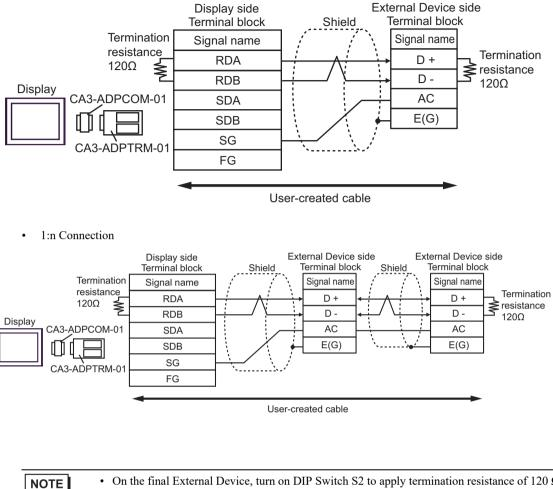
On the final External Device, turn on DIP Switch S2 to apply termination resistance of 120 Ω 1/2 W.
