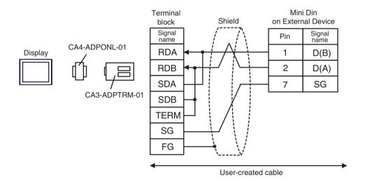
• The cable length must be 10m or less.
