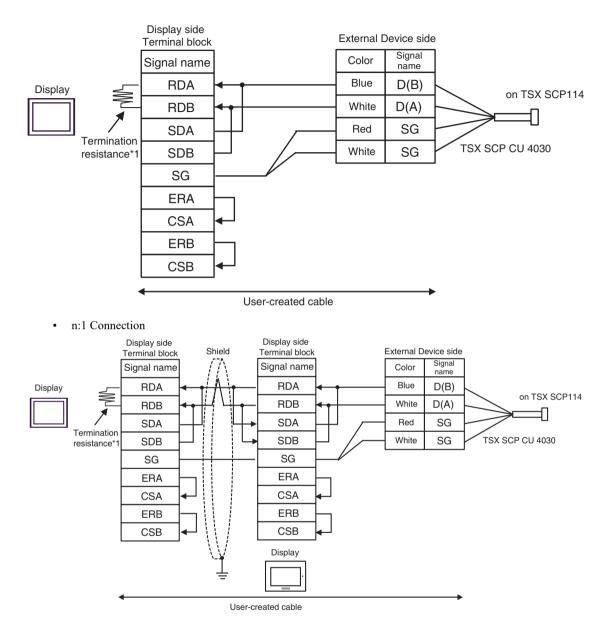
\*1 The resistance in the Display is used as the termination resistance. Set the value of the DIP Switch on the rear of the Display as shown in the table below.
