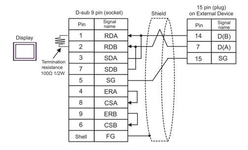
• The cable length must be 10m or less.
