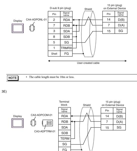
• The cable length must be 10m or less.
