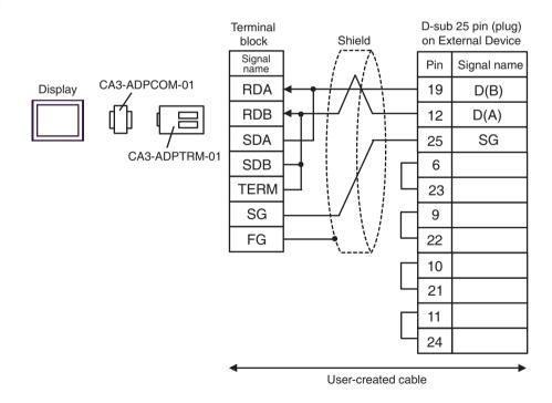
• The cable length must be 10m or less.
