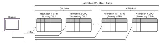
• 1:n Connection (Ethernet single/Netmation CPU single/dual mixed)
