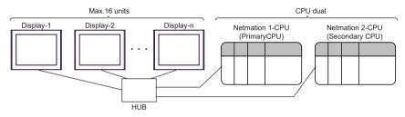
• n:m Connection (Ethernet single/Netmation CPU single/dual mixed)
