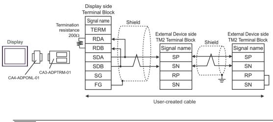
• Enable termination resistance by short-circuiting the terminatory External Device's RP terminal and the terminatory External Device's SN terminal.
