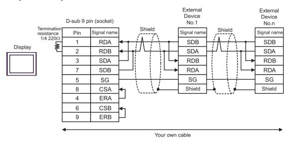
C) When using the connector terminal block conversion adapter (CA4-ADPONL-01) by Pro-face, the connector terminal block conversion adapter (CA3-ADPTRM-01) by Pro-face and your own cable
