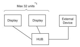
\*1 Number of connecting units is the unit number when connecting the display only. Number of connecting display will be limited by the number of other External Devices which is connected by Ethernet.
