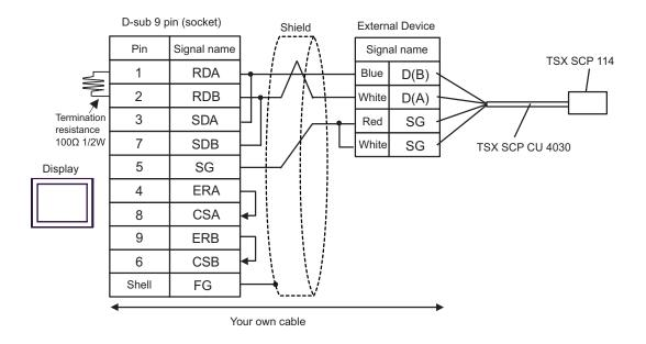
C) When using the online adapter (CA4-ADPONL-01), the connector terminal block conversion adapter (CA3-ADPTRM-01) by Pro-face, the Uni-Telway connection cable (TSX SCP CU 4030) and the PCMCIA card for RS485 (TSX SCP 114) by Schneider Electric
