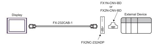
B) When using your own cable, the communication adapter (FX2NC-232ADP) by Mitsubishi Electric Corp. and the function extension board (FX1N-CNV-BD or FX2N- CNV-BD) by Mitsubishi Electric Corp.
