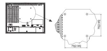
1) Attach one screw to the Display's rear side. Use a torque of 0.5 N•m to 0.6 N•m (4.4 lb-in to 5.3 lb-in).
