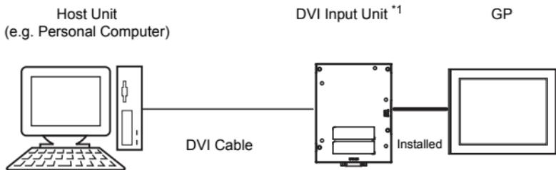
\*1 The Expansion Unit Interface 1 (EXT1) cannot connect an expansion unit when the DVI Input unit is connected to the AGP-35\*0T.
