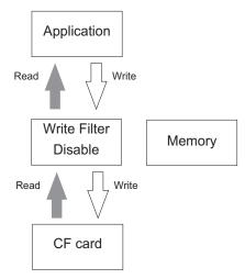
Turning OFF the power at the time of writing into CF card leads to data damage. When using this unit, use it with the Write Filter effective.Prevention of writing into the CF card is expected to prevent being damaged or prevent the CF card life cycle (Reference:  $0^{\circ}$ C -  $70^{\circ}$ C, Writing/Delete Times: 300,000 times per block) from declining as well.
