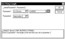
Obtains the length of the stored string. When a data buffer is assigned to Parameter 2, the number of characters up to the "NULL" character are stored in Parameter 1. (The NULL character is not included.)
