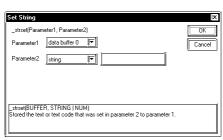
A fixed string is stored in the data buffer. A string specified with Parameter 2 is stored in Parameter 1.
