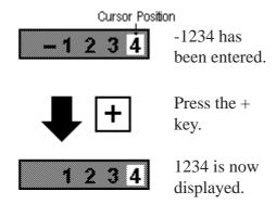
E.g. When the data format is "16-bit BCD" and the number of displayed digits is "4 digits," enter "-1" to store "F001h" in the data storage address using the key board on the touch panel.
