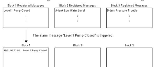
When the alarm message "Level 1 Point closed" is triggered, according to Display Mode settings (Block 1, Block 2, Block 3) of the Q-tag, the alarm message is displayed for the applicable tag. When the alarm message is triggered, it is stored in Block 1.
