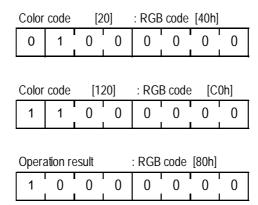
As a result of an XOR operation, overlapping color codes are "20" and "120", this overlapped color will be displayed as the following color code:
