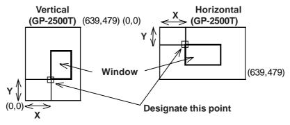
This function is only available with GP-2500T/2600T units that are equipped with the optional VM unit.
