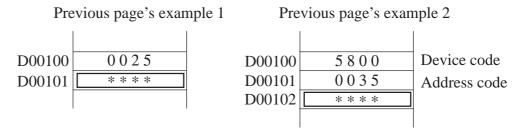
The range setting or arithmetic operation address will be D00101, which follows the Word Address D00100 in example 1. In example 2, the address will be D00102 because two word addresses, will be used for designating device and address codes. For the Range setting, the required addresses will be automatically allocated from D00101 or D00102.
