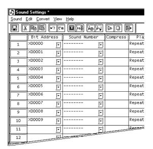
Automatic Address Allocation can also be performed via selecting the [Edit] menu – [Automatic Address Allocation] command. When a Symbol is designated as the Start Address, the added Address will be displayed as follows:
