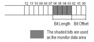
Set up the Bit Offset and Bit Length when portions of the Word Address are controlled elsewhere. It is necessary to set the monitor bits consecutively, as 00 - XX and YY - 15.
