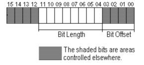
In the example above, the Bit Offset is 4 and the Bit Length is 8.
