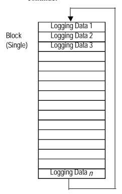
Same as the "Without Loop Operation", using loop operation, each logging data item also uses from 1 to 32 words.
