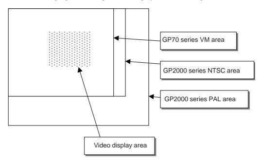
When the video display area is placed, the PAL area on the GP2000 series is clipped.
