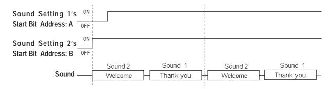
When 2 or more Start Bits turn ON at the same time, the sound items are normally output according to the sound setting's order. However, the output orders shown in the examples below may differ since the order of sound output can change due to the timing of the read out of the transmitted data.
