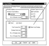
When there are multiple alarm screens, the Start Line must be "Display lines x number of Screens." On the first screen, the value is normally one, and increases by the number of rows set.
