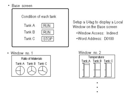
When the U-tag display window is set up as Indirect, the four consecutive word addresses beginning from the set word address will automatically be used for controlling the window display.
