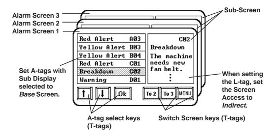
Enter the same address in the A-tag's Word Address (L-tag Word Address) and L-tag's Word Address. This example uses the GP internal LS area. Enter similar contents for Base screens 2 and 3.
