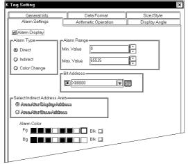
the word addresses which will contain the minimum and maximum values. These addresses will be automatically determined according to the setting of the Word Address designated on the Data Format page. For the Relative value input, the Output Range values designated on the Data Format page will be automatically designated as the minimum and maximum values. The possible values depend on the settings on the Data Format page.
