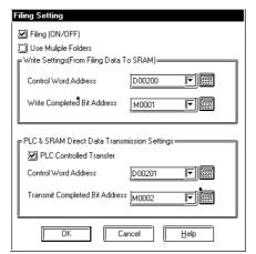
Write Settings (From Filing Data To SRAM) Control Word Address: D00200 Write Completed Bit Address: M00001
