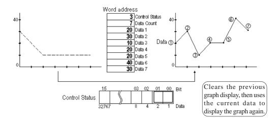
When "3" is entered to the Control Status word, both bits 00 and 01 turn ON, and after the graph display is cleared, the current data is used to display the graph again.
