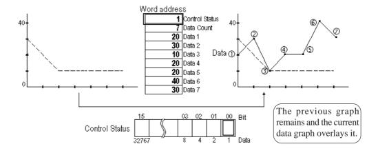
When "1" is entered to the Control Status word, bit 00 turns ON and the new graph overlays the previous display.
