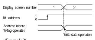
When the screen changes, the trigger bit value is 1, so the W-tag is activated and the data write operation is performed.
