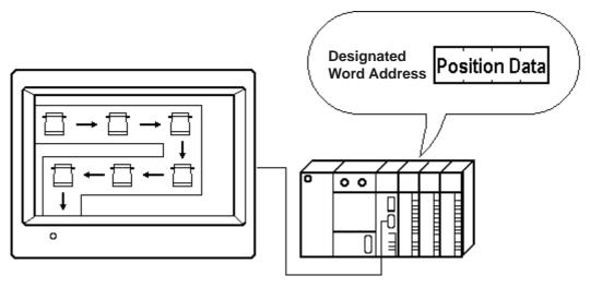
The positions for moving the Mark image are set on an R-tag. The position data refers to the position numbers designated in the R-tag.
