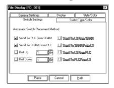
**Send To PLC From SRAM:** Selected **Send To SRAM From PLC:** Selected
