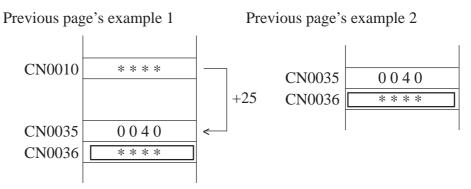
In both cases, CN0036 will be used for range setting and arithmetic operations. Addresses used will be allocated to the number of addresses designated by the Number of Ranges attribute.
