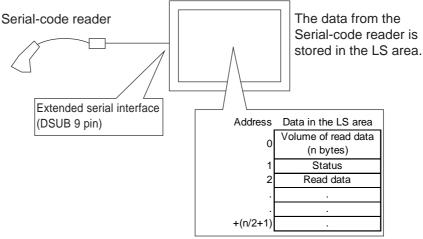
Note: Even if the Serial-code reader is set up, the serial 1-dimensional bar code reader can be also connected. However, the read mode should be set to "normal."
