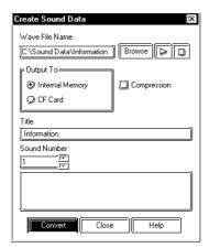
Click on the [Browse] button. Select a file to be converted or enter the file name. Then, select the data write destination and enter Title and Sound Number. To compress data after conversion via the [Convert] button, check the [Compression] check box.
