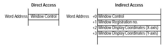
Each bit function for the Window Control is the same as in the Global Window. Set the Window Display Position's X-coordinate data in 8-dot intervals.
