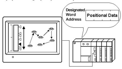
\*1. When a drawing or screen is used often, You can create the image on a Base Screen and register it, as a library item. The library's registered image is then displayed in the designated area, with the image's center point being placed at the desired position. This option is designated relative to a given start point.
