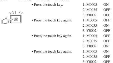
Each time the touch panel key is pressed, a bit on an address turns ON as follows:
