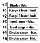
Indirect Designation "Area After Display Address Input/Display Designation "Indirect" No. of ranges: 3
