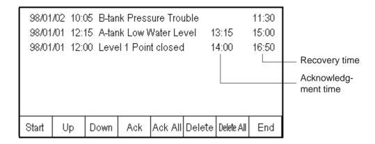
Pressing the Start key causes the cursor to appear. The cursor displays as a solid line over and under the current message. Other Q-tag select keys will not be enabled until the Start key is touched.
