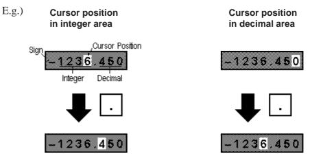
The cursor moves to the leftmost digit in the decimal area. The cursor moves to the rightmost digit in the integer area.
