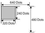
When an NTSC screen is displayed at 25% (1/4X magnification), it is displayed in the upper left corner of the screen. The remaining screen area will be displayed using the "Frame" color
