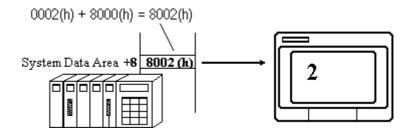
When the touch panel input has the highest priority for screen change, the screen change does not take place even if the same data is written to host (PLC) System Area +8 (as in step 6 of the previous page).
