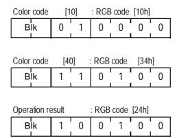
As a result of an XOR operation, when overlapping color codes "10" and "40", this overlapped color will be displayed as the following color code:
