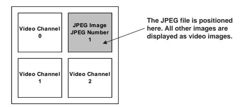
• Enter the image window number and the JPEG file number into the Video Control Area (Indirect Method).
