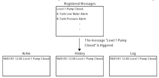
When the alarm message "Level 1 Point closed" is triggered, it is displayed according to Display Mode's settings (active, history, log) of each Q-tag.
