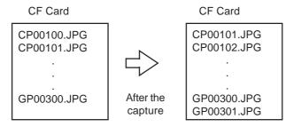
The file CP00100.JPG is deleted and the new file CP00301.JPG is created. However, if CP00100.JPG is a read-only file, the deletion is interrupted and "0101: CF Write Error" is set in bits 12-15 in the Status area.
