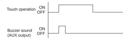
■ When the buzzer sound is ON, and the one-shot buzzer sound is OFF, the buzzer continues to sound while the touch panel switch is depressed.
