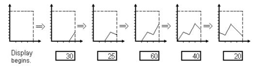
When the sampling period is designated as 1 second, depending on the size of **Note:** the graph area used, graph scroll processing can take almost one second, and communication and tag processing can be affected. In this case, setting the sampling period to 2 seconds should correct the problem.
