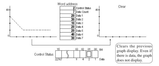
When "2" is entered to the Control Status word, bit 01 turns ON and the new graph display is cleared.
