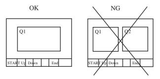
◆ Set the Q-tag select keys to the same screen that the Q-tag is set to. They cannot be used if they are set to a screen that the Q-tag is not set to.
