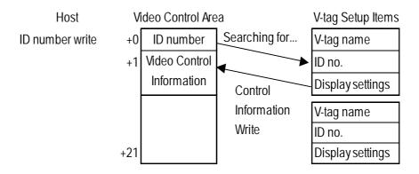
It is unnecessary for the host (PLC) to receive a large amount of video control data at the start, since the video display begins with just the setup ID number. Each ID number's control information (setting items) can be collected in the GP, thereby reducing the load on the host (PLC).
