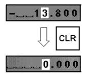
The integer and decimal sections are cleared to zero as the integer part is reduced to a single digit, the zero in the unit position. The cursor appears in the lowest integer position.
