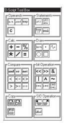
The buttons in the tool box are classified and positioned by each function group.
