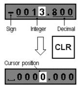
The sign is replaced by a blank space, and the rest of the numbers are cleared to zero. The cursor appears in the lowest integer position.
