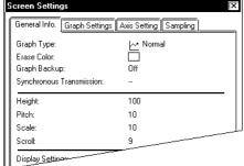
To check the current settings, display the trend graph screen and select the "Tag" selection's "Setup Screen".
