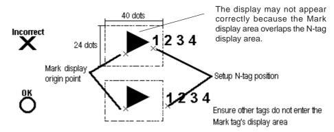
• Overlapping the Mark's rail position with other tags causes an incorrect display.
