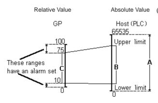
(1) Displays the range [A] as a percentage. Data in the 10 - 75% [B] range is displayed as normal data, and data outside this range is displayed in alarm mode.
