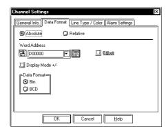
To check the current settings, display the trend graph screen and select the "Tag" selection's "Setup Channel".
